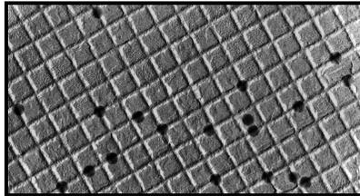
1. To calculate the electron microscope magnification using the pattern of the **diffraction grating replica**: Take the measurement, in millimeters, between the limiting lines of as many squares of the replica pattern as possible. Apply the following formula:
